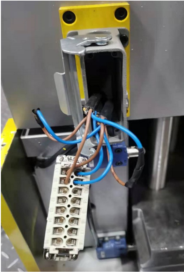
Connections of limit switch with connector plug
